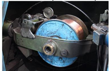
High speed buncher for production of flexible bunches from multiwire bobbins.
